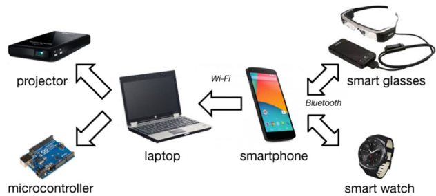
Figure 8. The candid interaction ecosystem links mobile and wearable devices to a laptop computer, which operates microcontrollers and projectors in our prototypes.
