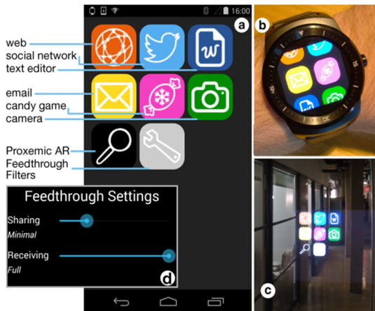
Figure 7. Our homogeneous platform has a similar look and feel on the (a) smartphone, (b) smart watch, and (c) smart glasses. (d) Feedthrough sliders control the extent of information sent and received about device activity.
